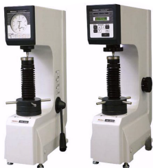
TESTER FOR ROCKWELL HARDNESS
